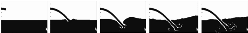
Fig. 9. The jet falls into the pool. Effect of “shaggy head” is eliminated.
