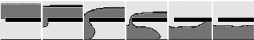
Fig. 4. Water flow from floor to floor through a hole. Heavy viscous incompressible fluid (Continuous marker function).
