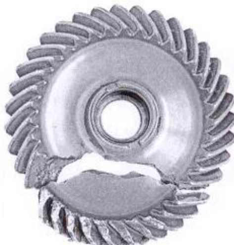
FIG. 1: View of the destroyed gear after 39 cycles of starting and stopping the gearbox.
