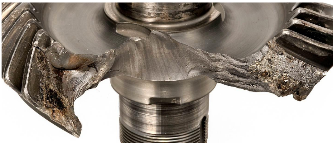
FIG. 2: View of the fracture of the gear wheel of the gearbox of the PS-90A engine.
